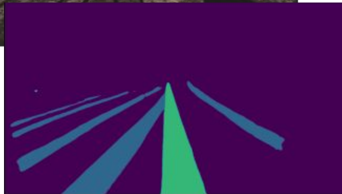
Top: image from camera placed on locomotive Bottom: regions of main (green) and side railways (blue)
